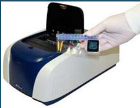
Figure 1. Respiratory virus panel (RVPCR) testing instrument. One specimen per instrument can be utilized at a time.
